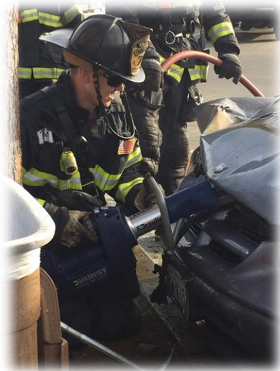
Extrication tool used to access a fire in the engine compartment.
